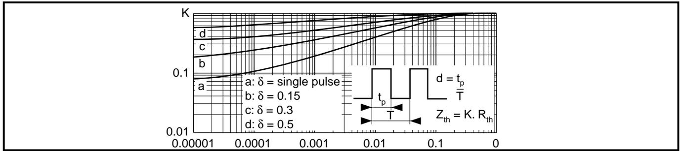
Fig.2 Typical transient thermal impedance
