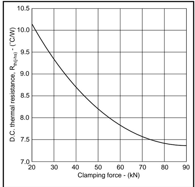
Fig.2 DCR1674SZ thyristor - variation of R<sub>th</sub> with load
