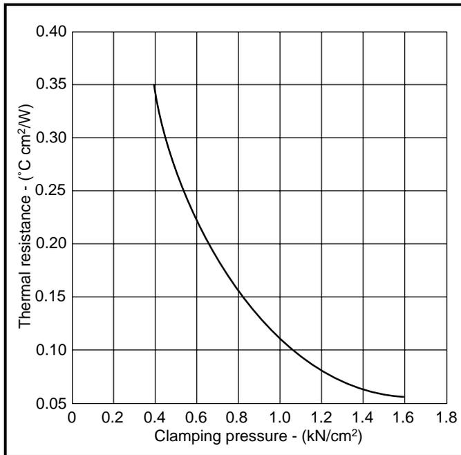
Fig.1 Additional thermal resistance for dry interfaces of a FFS thyristor
