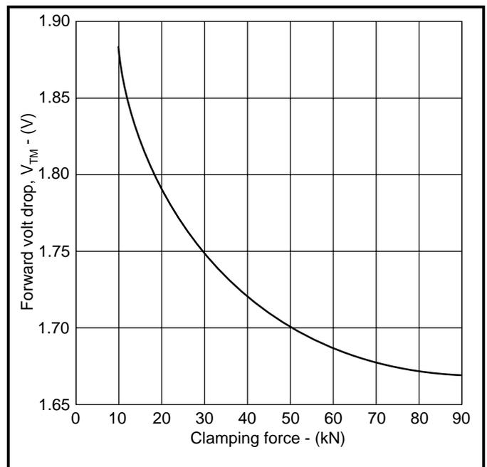
Fig.3 DCR1674SZ thyristor - variation of V<sub>TM</sub> with load
