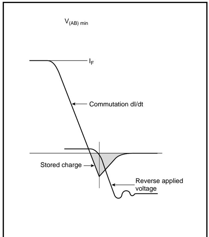
**Fig.4 Commutation waveforms**
