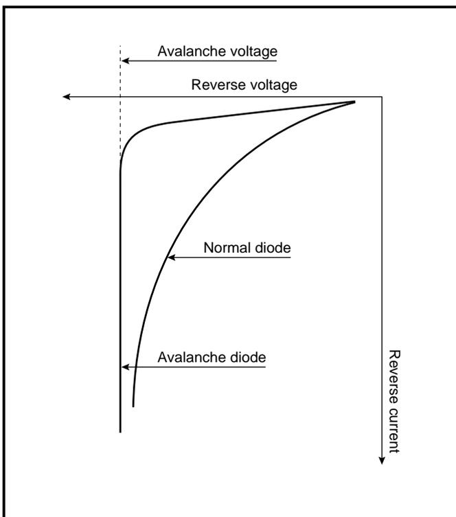
**Fig.1 Reverse characteristics**
