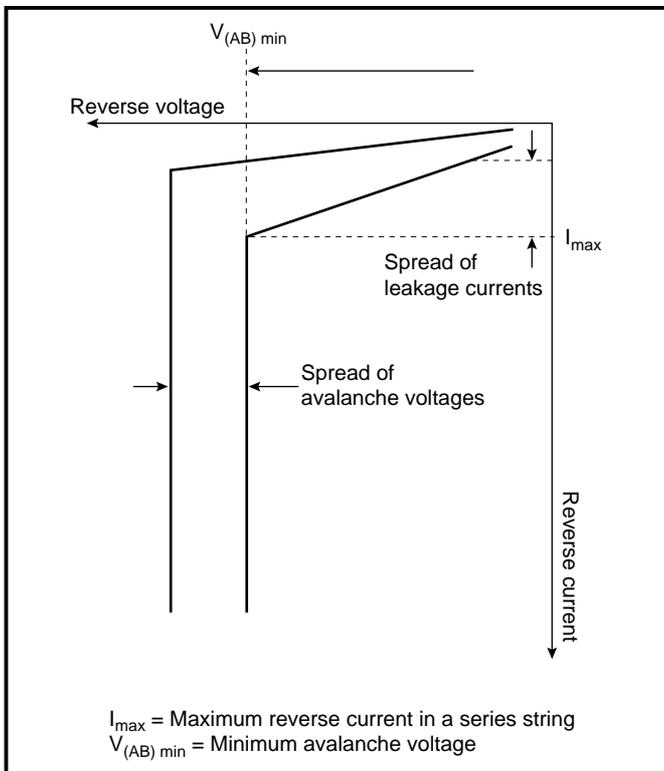
**Fig.3 Spread of reverse characteristics**
