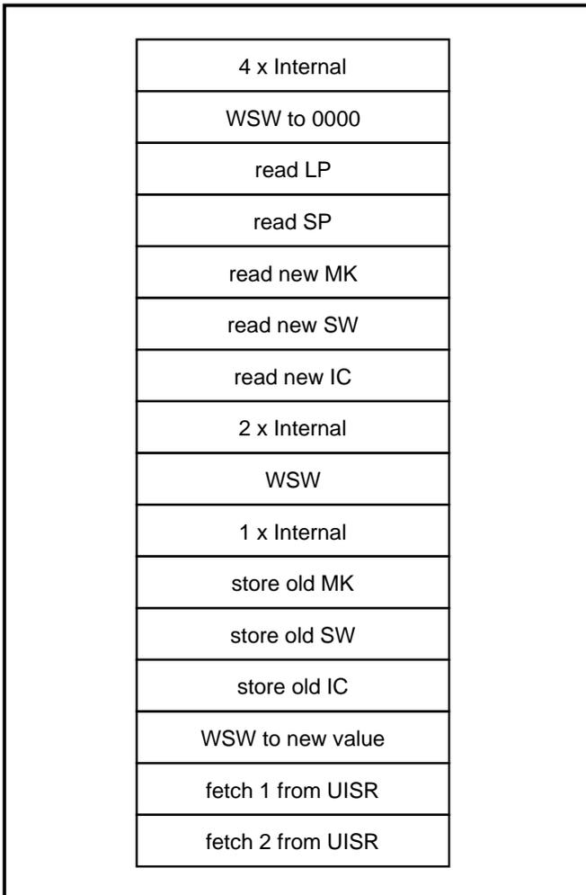
**Figure 6: Machine Cycle Description
