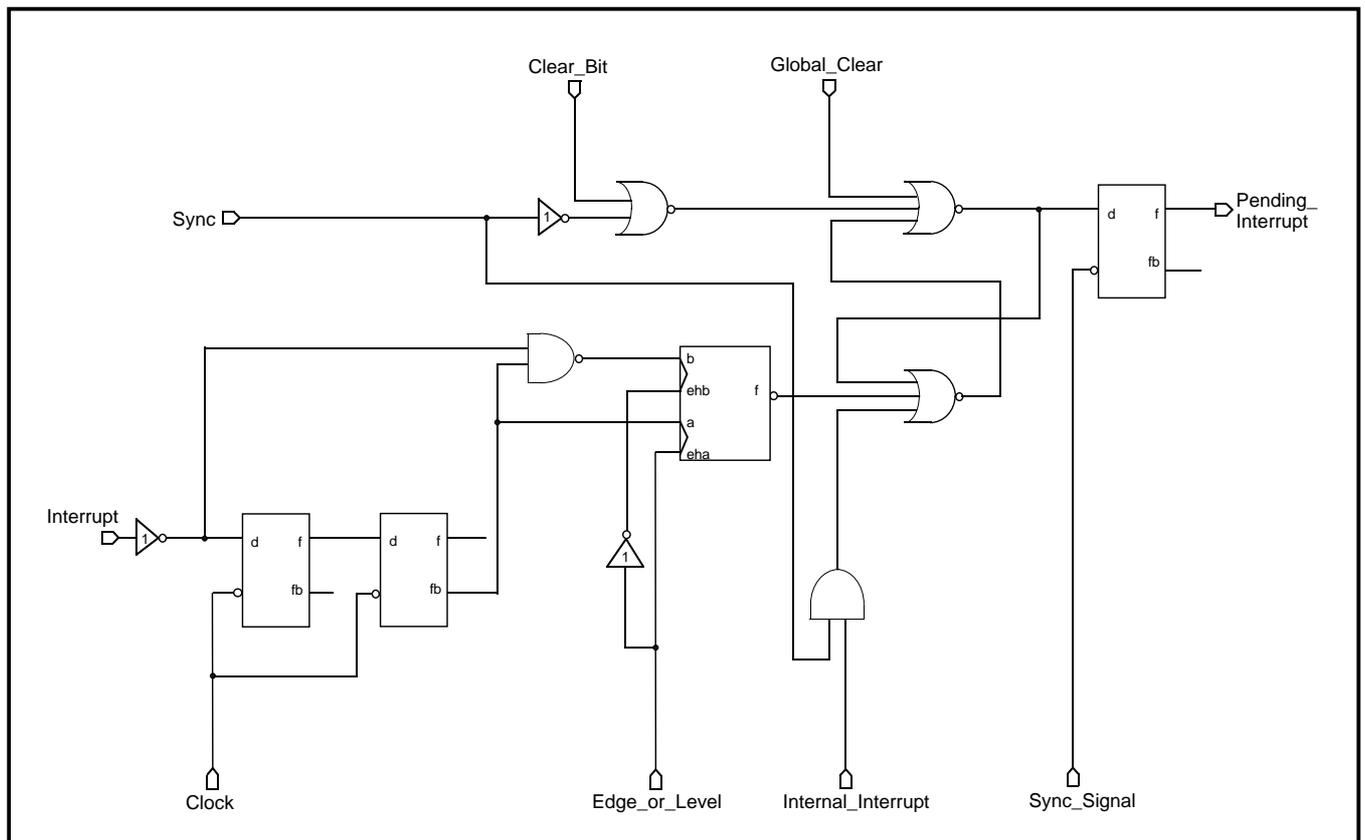
Figure 1: Edge and Level Interrupt Latching Circuit
