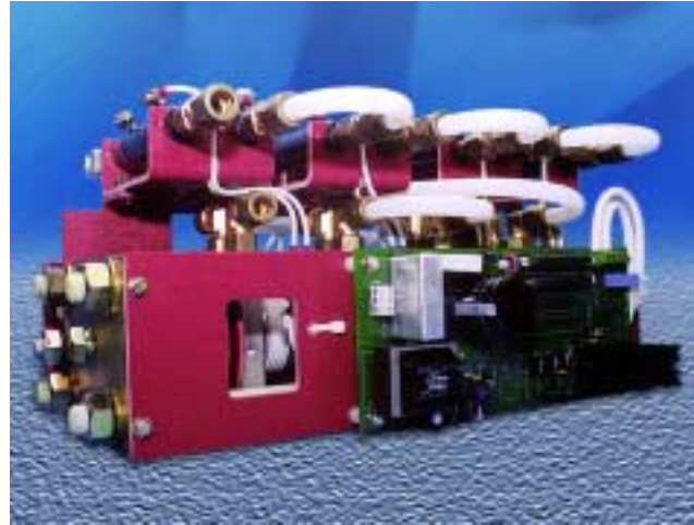
Liquid cooled thyristor assembly incorporating gate firing circuitry
