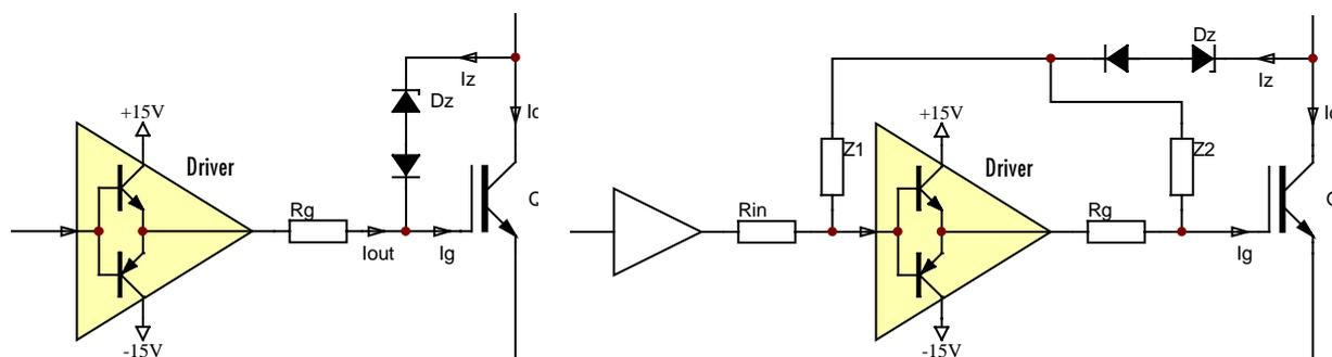
Fig. 6 Basic Active Clamping circuitry (left) and advanced circuitry used in SCALE HVI drivers (right)
