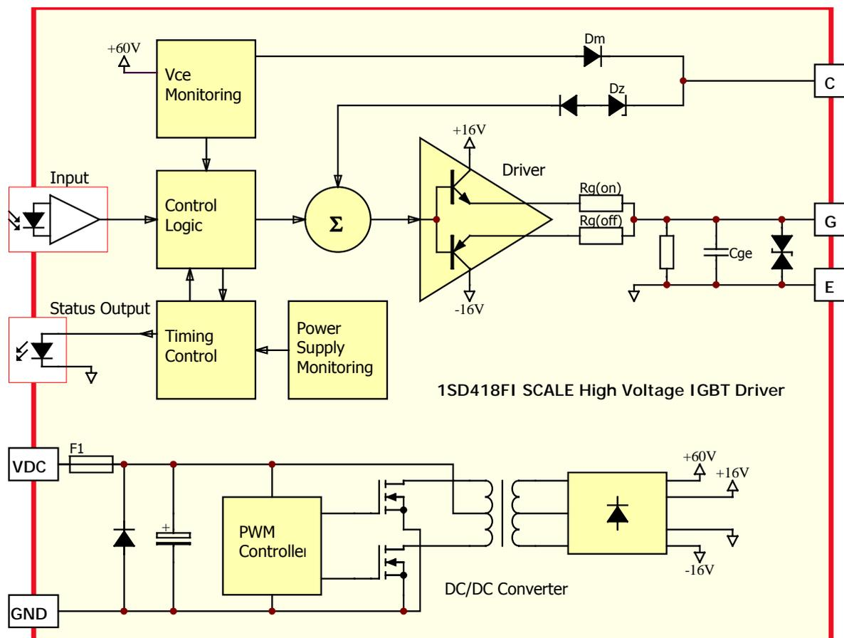
Fig. 3 Block diagram SCALE HVI driver
