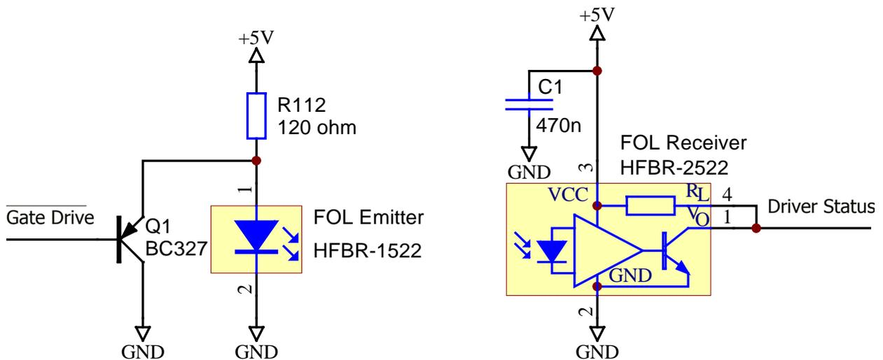
Fig. 11 Recommended circuitry for the fiber optic links
