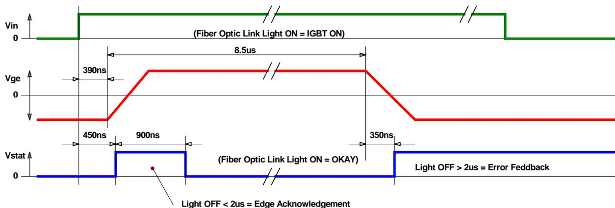
Fig. 10 Failure status feedback; signals under short circuit conditions
