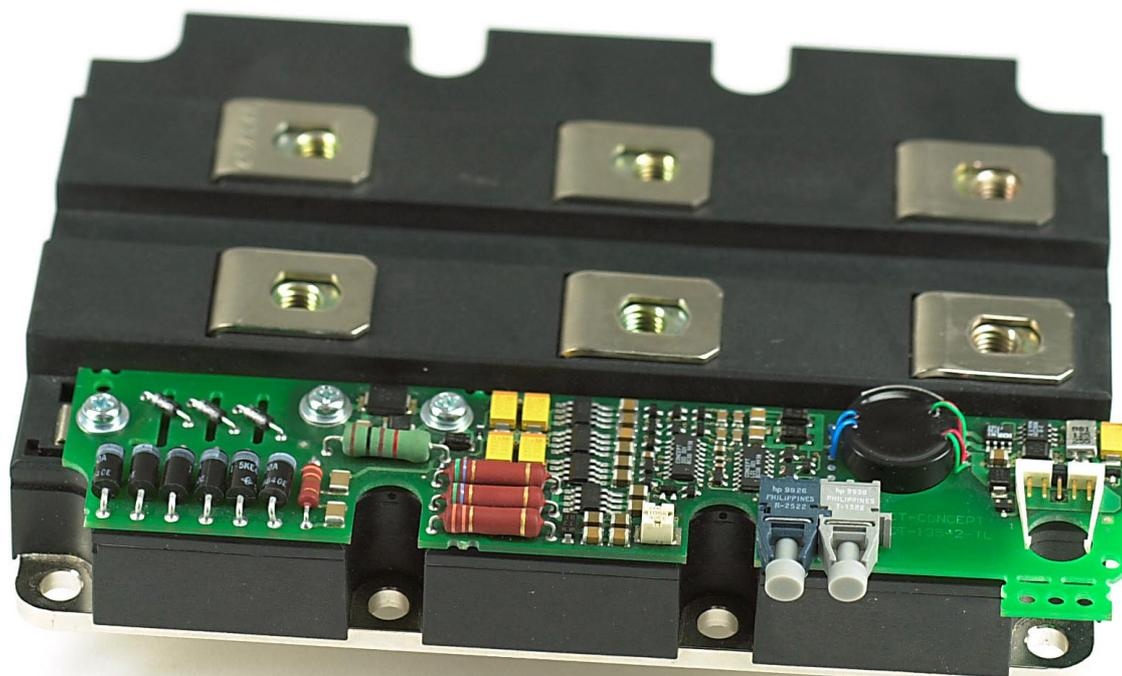
*Fig. 1 SCALE HVI driver 1SD418FI screwed onto a IGBT 1200A/3300V*
