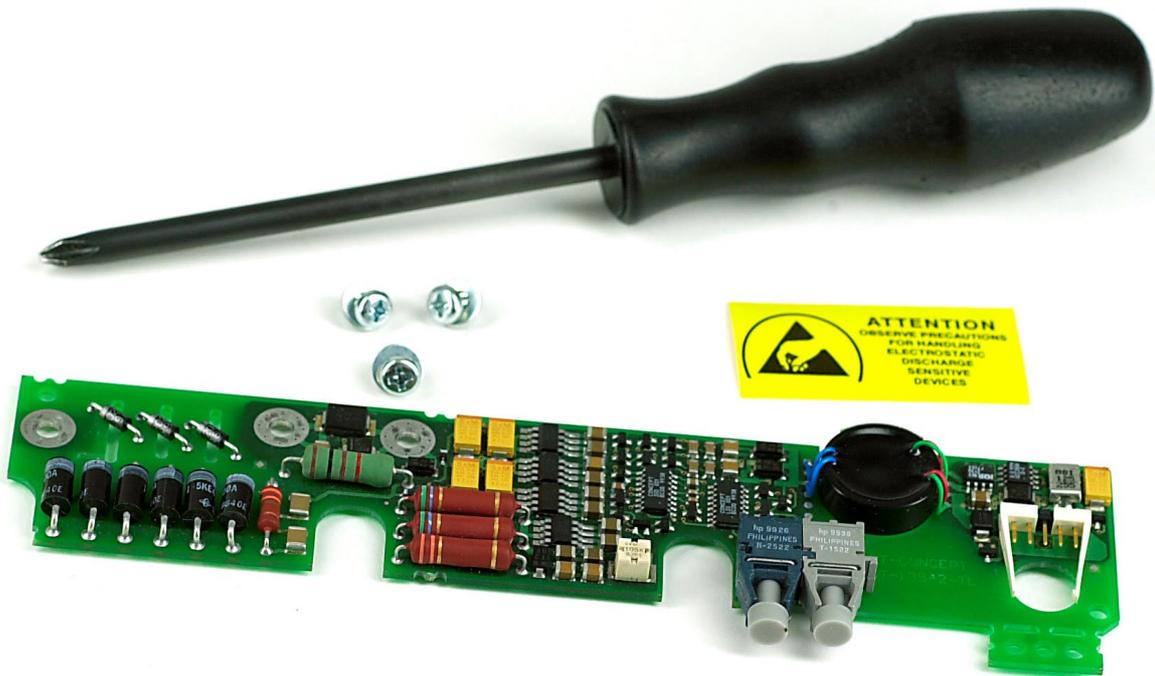
*Fig. 2 SCALE HVI driver and the needing tool*
