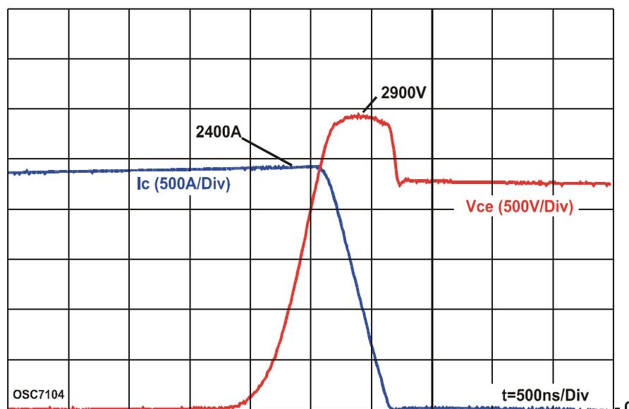
Fig. 7 Behavior of a 1200A/3300V-IGBT for turning-off a collector current of 2400A, which is twice the nominal collector current
