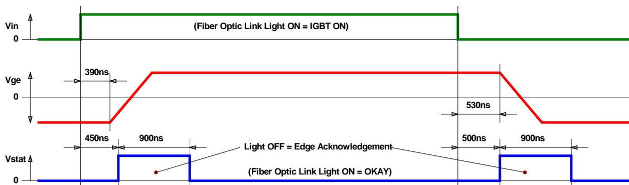
Fig. 9 Failure status feedback; signals for normal operation
