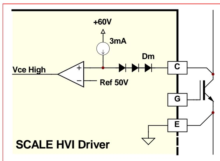
Fig. 4 Vce-desaturation monitoring
